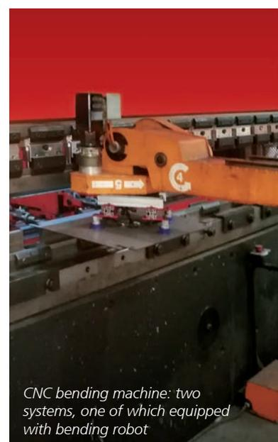
CNC bending machine: two systems, one of which equipped with bending robot
