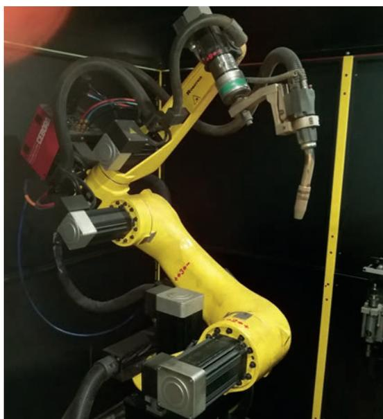
Left: a robot for welding telescopic table supports, revolving seat base plates, and parking feet
