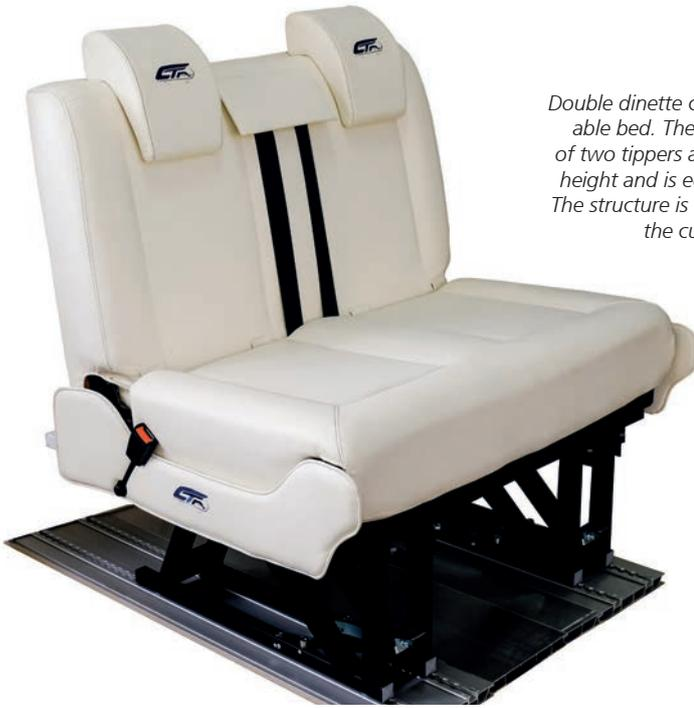
*Double dinette converting into a comfortable bed. The Dinette Sleep is made up of two tippers and headrest adjustable in height and is equipped with safety belts. The structure is tested in accordance with the current European standard.*
