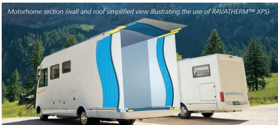
Motorhome section (wall and roof simplified view illustrating the use of RAVATHERM™ XPS)
