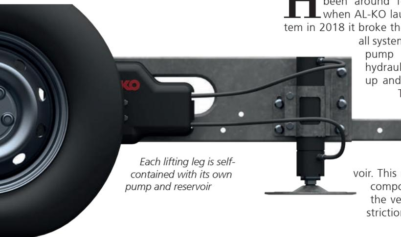
Each lifting leg is self-contained with its own pump and reservoir
