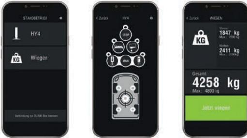
The levelling screen (centre) also contains the functions for night time tilting and tank emptying.
