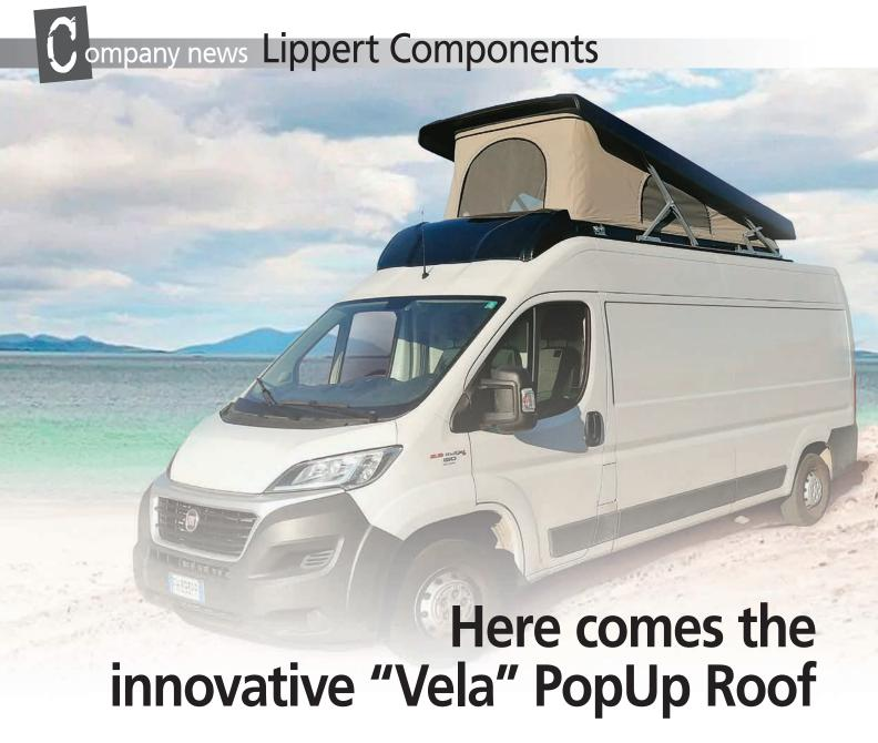
Available from this September, the new "Vela" PopUp Roof from Lippert Components, developed and produced in Europe, is sturdy and light, weighing 20 to 30 percent less than comparable fibreglass products. It provides a real extra bedroom for campervans with a double bed measuring 200 x 130 cm, and is built with a thermoformed twin sheet technique plus an exclusive, patented solution for channeling hot or cold air.
