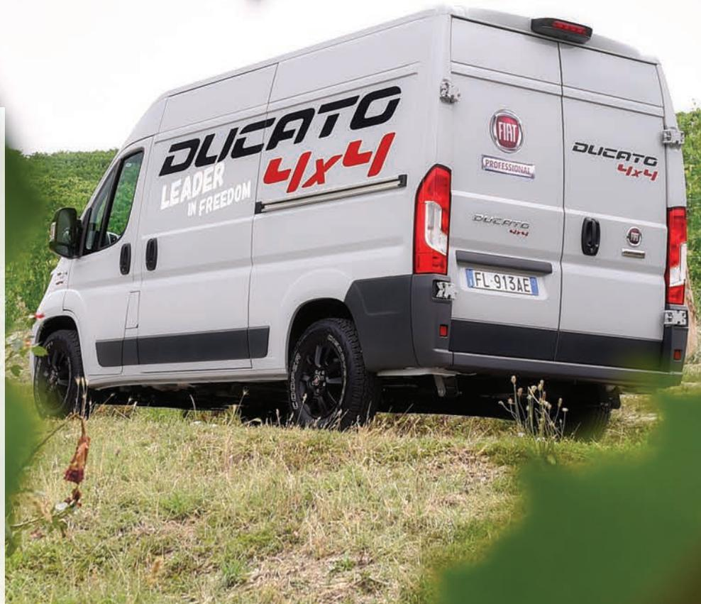
A revolution that seems to have no end. The current, and sixth, generation offers the highest gross vehicle weight in the segment, the highest front axle load (up to 2100 kg) and the highest rear axle load for vehicles with single-wheel rear axles (up to 2500 kg), as well as the highest maximum payload. The current generation of Ducato, called the X290, boasts the highest total ground weight in the segment: up to 4400
