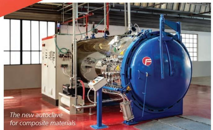
The new autoclave for composite materials
