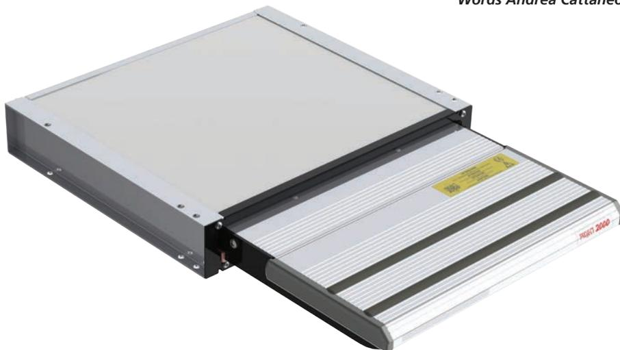
engine is water-proof, featuring a built-in thermal protector. The sliding on special guide is patented and allows a smooth sliding even after a long period of disuse. The waterproof "open step" sensor was inserted into the motor unit to guarantee safety and prevent damages. The footboard is made of anodized aluminium with a non-slip rubber
